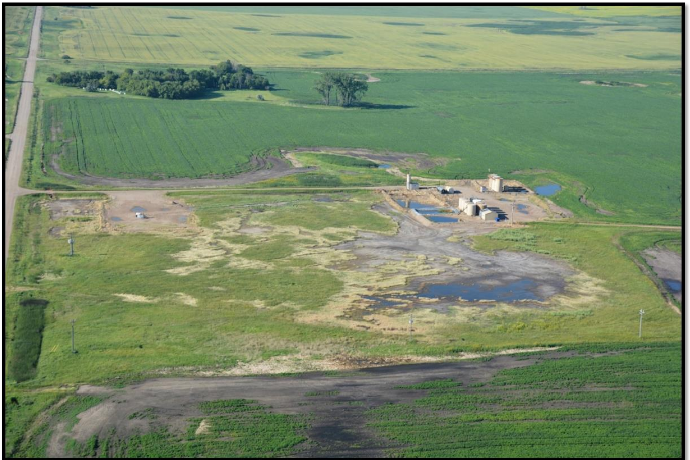
Well #15288 - Note the barren soil emanating from the well site. Duke University took water samples from standing water in the road ditch (far left hand side).
