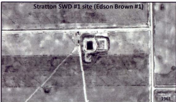
The site contained two brine holding ponds from 1959 to at least 1970 (with dimensions of 100 x 90 ft and 60 x 100 ft and 5 feet deep). This well produced 178,000 barrels of saltwater.
