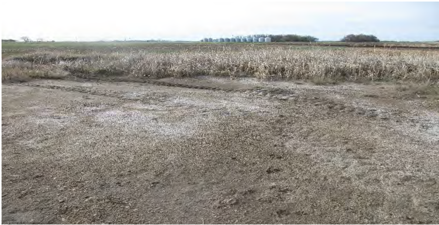
Photograph facing south from an oil & gas facility showing the visually impacted area, which measured approximately 40 feet by 15 feet. The area showed a lack of vegetation and salt crusting and lies directly north of a wetland.
