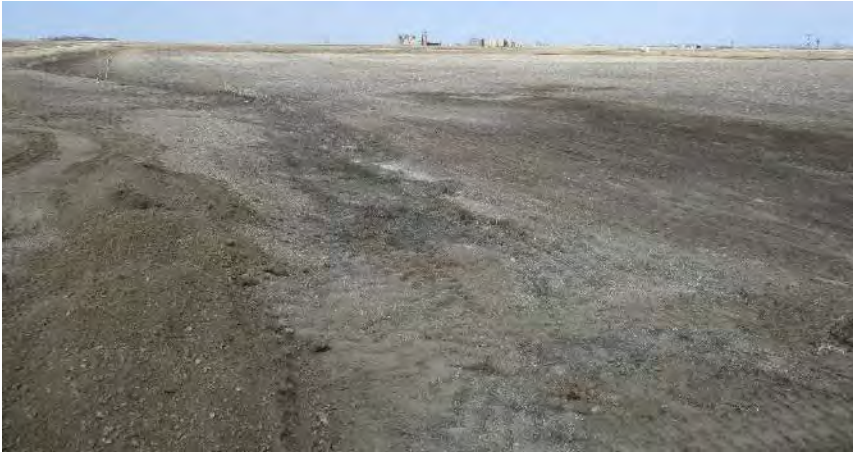
Photograph facing west off of an oilfield lease road showing stressed vegetation, dead zones, and salt crusts at the site.
