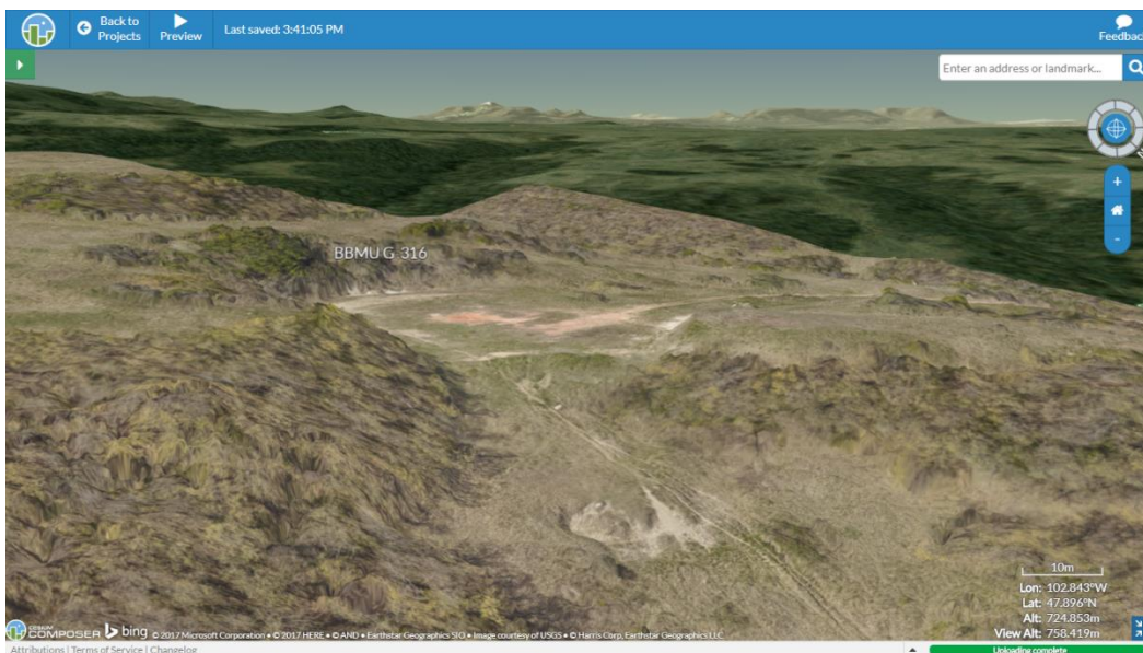
Figure 46: High resolution imagery and DTM of G-316 looking to the south west. The imagery suggests that the excavated soil was pushed down the slope at the front of the image (North East).
