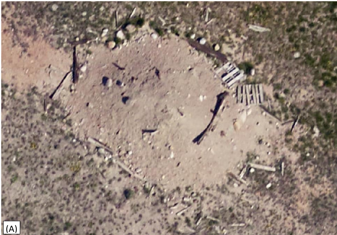
Figure 33A: Visual detection of multiple debris piles in RGB imagery at 3-cm resolution are clearly visible at modest image enlargement (image not maximum zoom)
