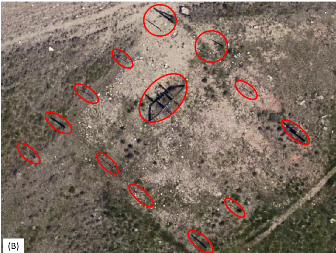
Figure 34B: Visual detection of piping infrastructure of various sizes in RGB imagery at 3-cm resolution are also clearly visible at modest image enlargement (image not maximum zoom).
