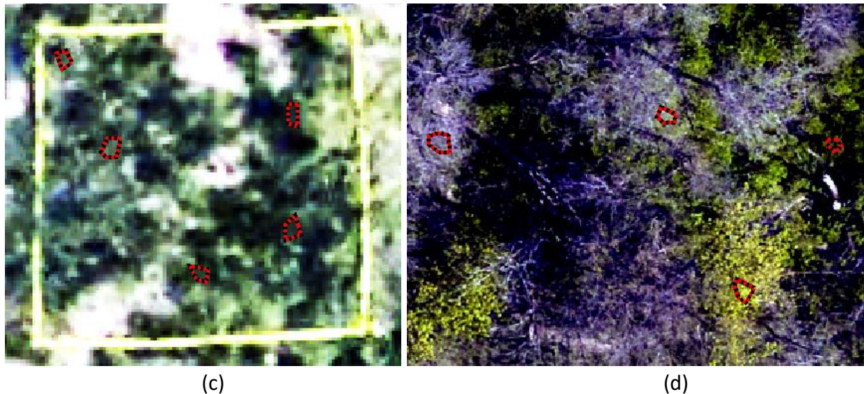
Figure 23: Example of training set selection for Bare Soil (a), Weed (b), Grass (c), and Wooded areas (d). The training sets must be representative samples for each land cover class in the image. Notice the high spectral variability in the wooded (forest) class.
