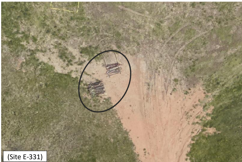
Figure 35: Infrastructure detection in an intermediate restored site (E-331); pipes and debris have been picked-up from the site and stockpiled, but have not yet been removed from the site
