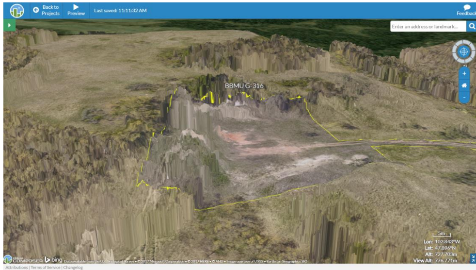
Figure 43: High resolution imagery and DTM of G-316. Vegetation (trees and shrubs) is represented as surface features.
