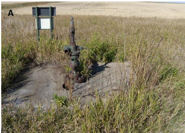
Figure 10: TMU F-144 residual infrastructure ranging from the wellhead to rig anchors. Overall the site was in good vegetative state and surrounding land was being used for production.
